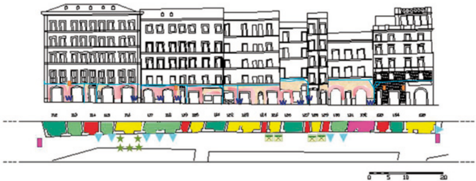
Fig. 9 - State of conservation of the ground floor facades and related functions, along Via dei Pastini.
